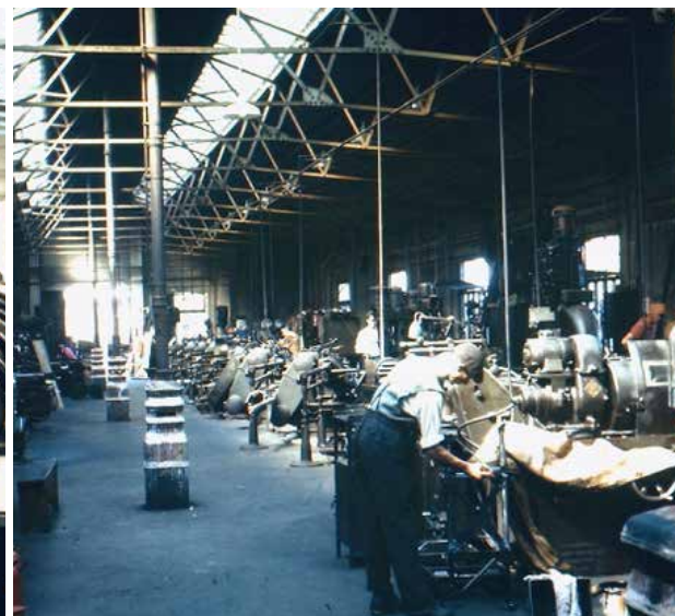
Forming panels in the sheet metal shop 2
