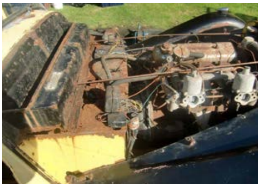
Engine bay of chassis number 6428 showing the Derrington four-branch extractor exhaust system. Courtesy of Bill Hayter, Vancouver, BC.
