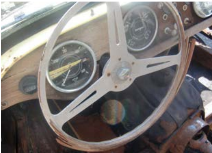
Dashboard from chassis number 6428 showing the knob to alter the Armstrong 'Selectaride' rear shock absorbers. Courtesy of Bill Hayter, Vancouver, BC.
