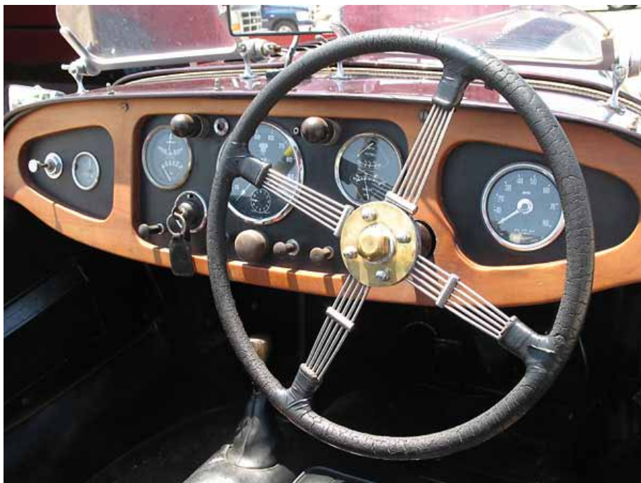
An Ashby "Brooklands" steering wheel in a 1938 Series 1 4-4. (© BritishRacecar.com)
